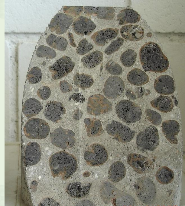
Concreto leve com argila expandida
